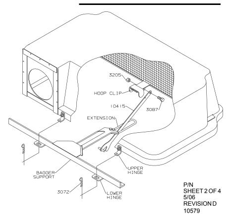
11) To adjust the grass catcher top latch, both grass catcher bags must be in place on bag frame. With grass catcher top closed, slide the center support extension (2864) horizontally until it contacts the catch handle (2887). Adjust the catch handle vertically until it contacts the center support extension. This adjustment should allow the top to close with ease and fit tightly when closed. Minor adjustments may be required to achieve proper fit. <u>Tighten all grass catcher hardware</u>.
